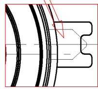
10. Remove the special timing tool, and mount the valve cover, the high voltage ignition cable and the timing belt cover.
