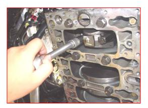
6) Remove the connecting rod bearing lower cover.
