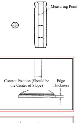
e: Check the valve seat insert.
