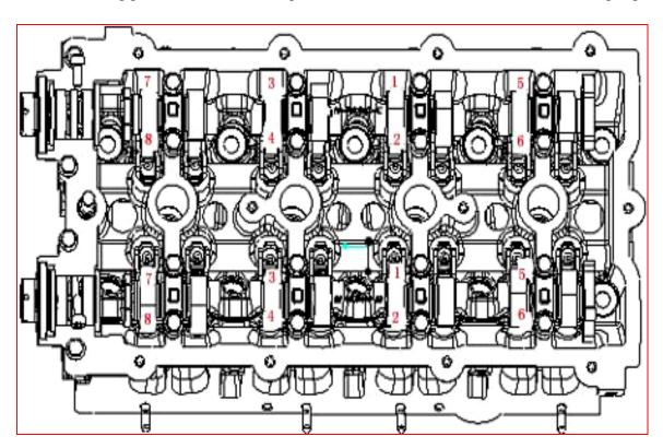
See the following picture for removal sequence of intake and exhaust camshaft-bearing caps:
