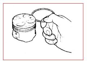
b. Examine the clearance between piston ring and ring groove with feeler gauge.
