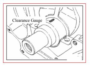
d): Mount the main bearing cap carefully and screw down the bolt with specified torque.
