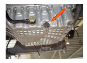
2) Use 10#open end wrench and 10 # sleeve to dismantle the fixed bolt of oil pan (18 M7 $\times$ 25, 3 7 $\times$ 40 and 4 M7 $\times$ 95).
