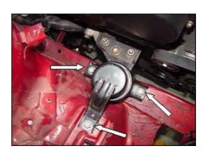
16. Dismantle the hexagonal flange bolts of left suspension cushion in order to ensure no connection between the engine and car body. Lift down the crane carefully and shift out the power assembly.
