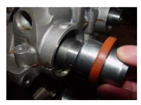
4) Press the oil seal into the oil seal seat ring carefully, and use hammer to knock it to the specified position.
