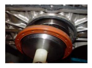
2) Apply a layer of oil onto the front oil seal lip of crankshaft equally. Fit the oil seal onto the special tool, and then press it into the oil seal seat ring.
