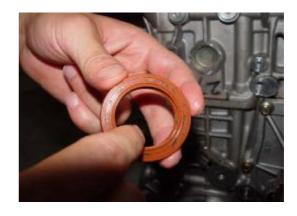
3) Fit the lubricant-applied new oil seal into special tool.
