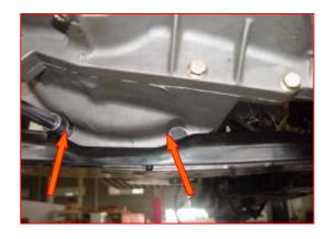
4) Use 15# sleeve wrench to dismantle the bolts connecting the oil return pipe of PVC valve and oil pan
