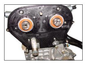
7) Dismantle the air intake and exhaust camshaft bearing caps in turn, and place them well in order.
