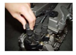
3) Use 10# sleeve to dismantle the fixed bolts of ignition coil.
