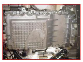
3) Use 17# sleeve wrench to dismantle the bolts (2 pieces, black) connecting the oil pan and transmission housing.
