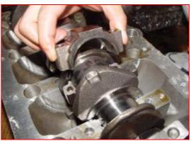
7) Use wood stem to uplift the connecting rod and piston slightly, and then dismantle the piston and connecting rod assembly.
