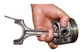
5) Mount the connecting rod lower bearing and connecting rod cap together, and apply engine lubricant onto the bearing.
