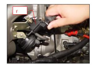
6. Dismantle (g) the earth cable bolt of cylinder head, remove (h) the wire harness plug of starter coil, (i) wire harness plugs of four oil injectors, (j) knock sensor plug, (k) wire harness plug of throttle valve controller.
